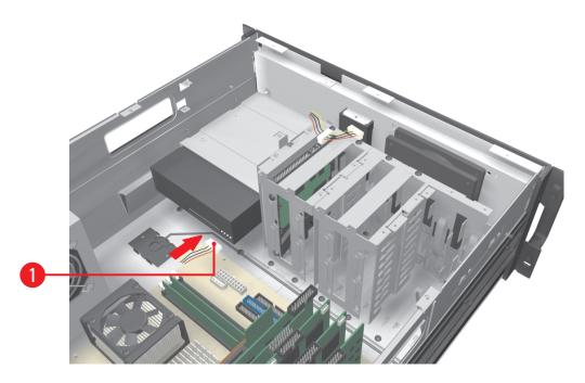
Figure 13. Installing the DVD-RW Power Connector
